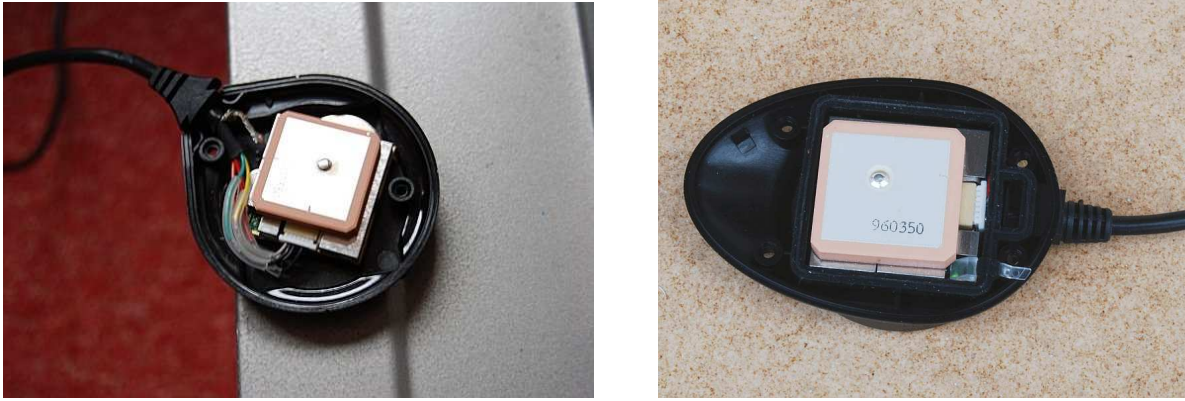
Figure 29: An EM-406A module embedded into the housing of a Fortuna U2, to the left, and embedded into a housing of a Navilock NL-303P, to the right.
