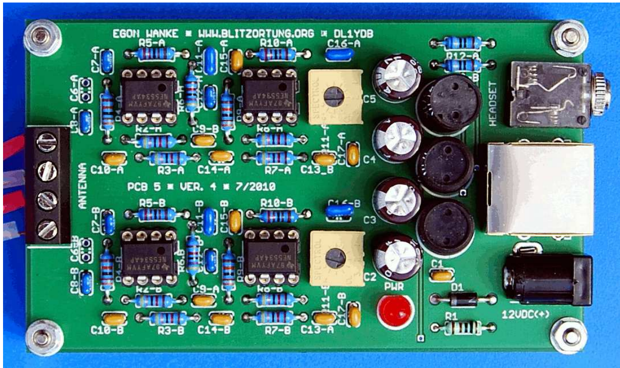
Figure 13: The assembled pre-amplifier PCB 5 Version 4.
