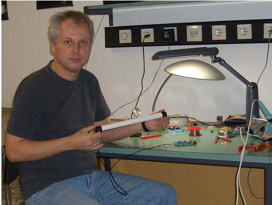
Figure 8: A 35 cm ferrite rod antenna in my hands.
